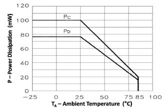
Fig 1 Power Dissipation vs Ambient Temperature
