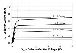
Fig 3 Collector Current vs Collector-Emitter Voltage
