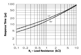
Fig 6 Response Time vs Load Resistance
