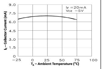
Fig 4 Collector Current vs Ambient Temperature
