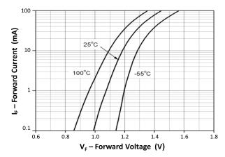
Fig 3 Forward Current vs Forward Voltage
