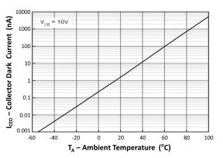
Fig 4 Collector Dark Current vs Ambient Temperature
