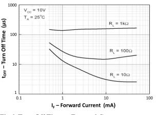
Fig 6 Turn Off Time vs Forward Current
