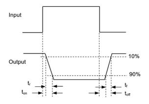
Switching Time Test Circuit and Waveforms
